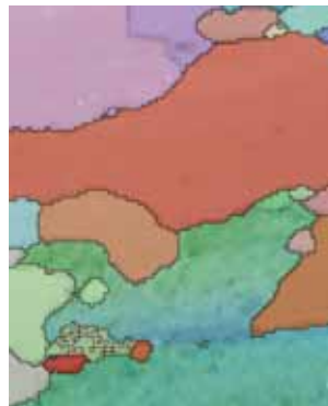
Fig B—The different colours in this lower-magnification image represent crystals in the alloy. The crystals shown are about the width of a human hair.
