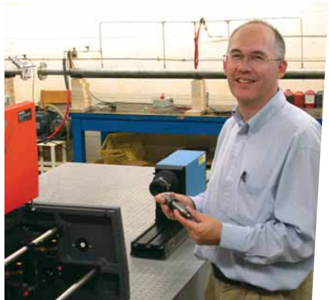
Martin Davy uses equipment provided by CFI funding for his clean energy research. The laser is used to excite fluorescence in fuel that is then photographed.
